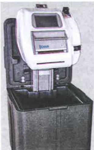
Fig. 19.1: Portable dialysis unit (NxStage System One) with the box for transport.
